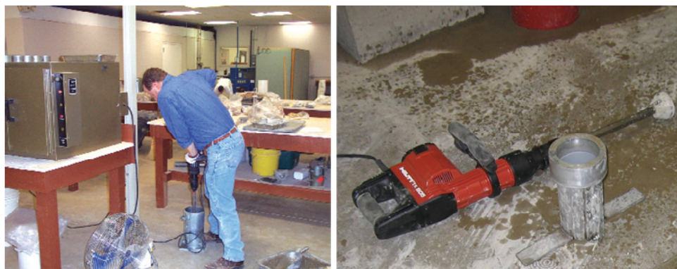
Figure G-14 Compacting hammer for RCC
