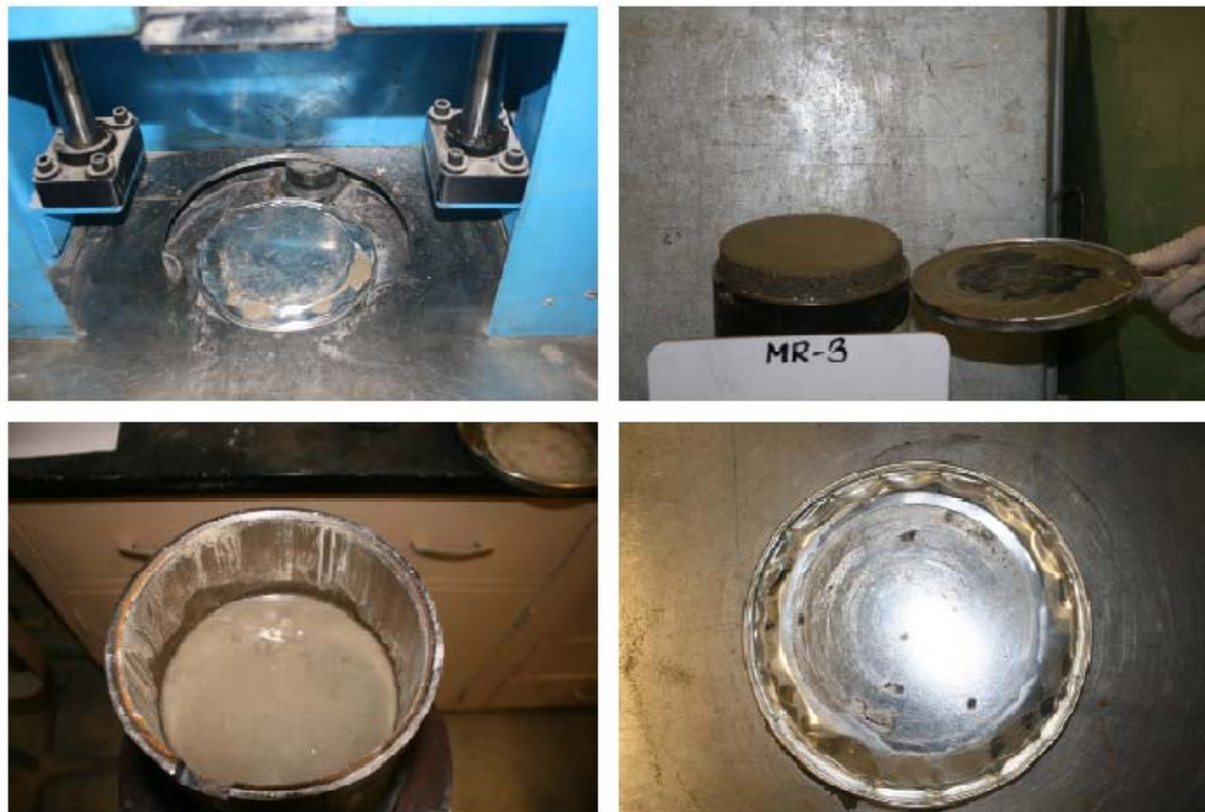
Figure 6-10 Gyratory compactor: squeezing out of paste
