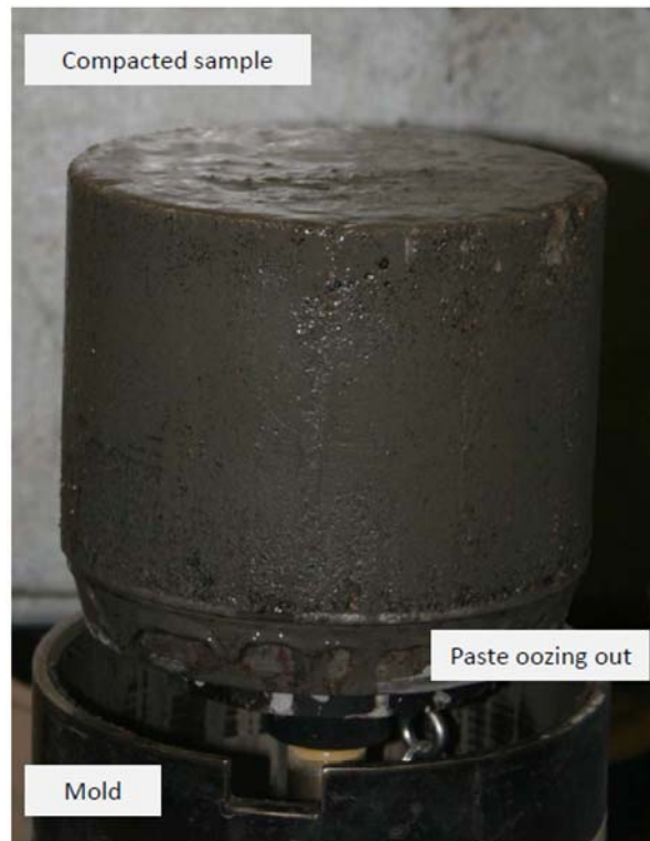
Figure H-30 Paste oozing out from the gyratory compacted sample
