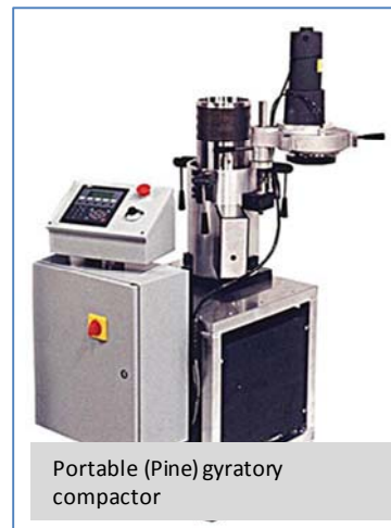
Figure E-1 Gyratory compactors (taken from the personal collection of the author and [12-13])
