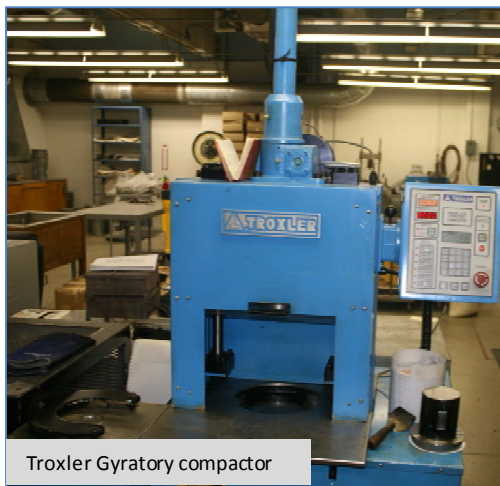
Figure E-1 Gyratory compactors (taken from the personal collection of the author and [12-13])
